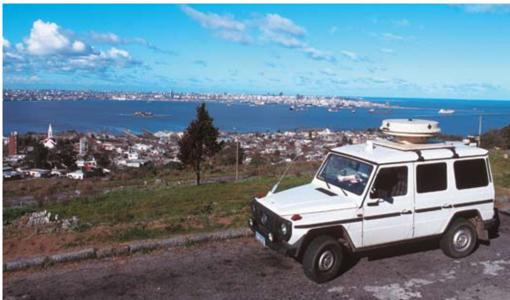
R&S®ADD295 mounted on a vehicle roof
